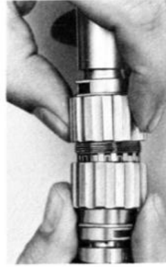
Figure 3-2. Mating of Type 900-BT connectors.
